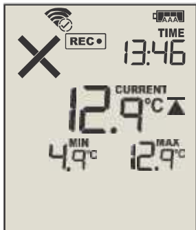
Recording - Upper Alarm.
